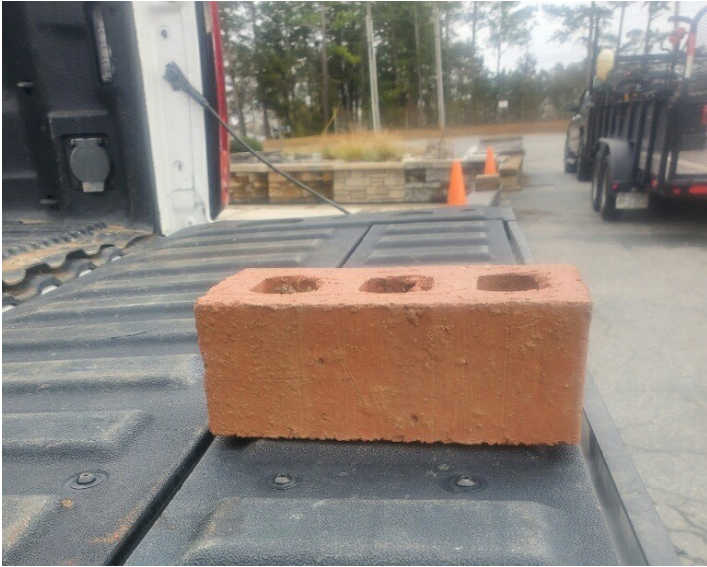
This color brick will be used for the whole project. We are having it made to match existing brick.
