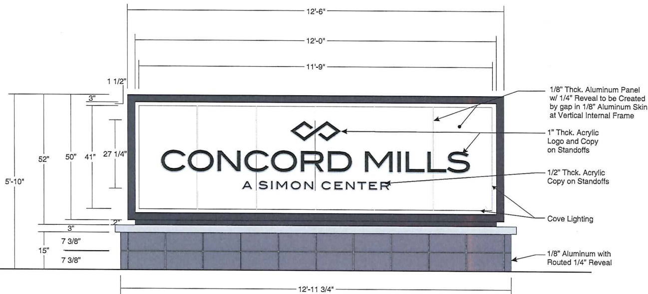
1 FRONT ELEVATION TEMPORARY SIGN 12.1 SCALE: 1/2" = 1' - 0"
