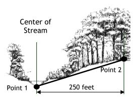
Pre-development elevation of Point 1 in feet =  $E_1$ Pre-development elevation of Point 2 in feet =  $E_2$
